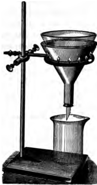
FIG. 4 HOT-WATER FILTERING APPARATUS WITH RING BURNER.
